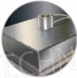
Saldatura a mezzo pistone pneumatico 3 ATA Sealing by pneumatic piston, 3 Ata
